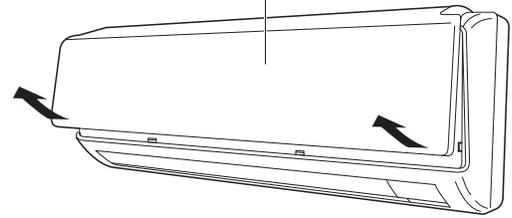
2. Remove the filter attached to the rear of the air intake grille.
