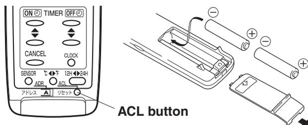
1. Slide the cover in the direction indicated by the arrow and remove it.
