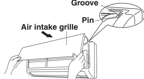
3. To attach the air intake grille to the indoor unit, press its bottom right and left corners as well as its bottom center into place.
