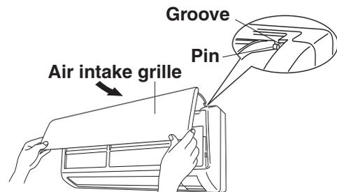
3. Press in the bottom right and left corners of the air intake grille to attach the indoor unit.
