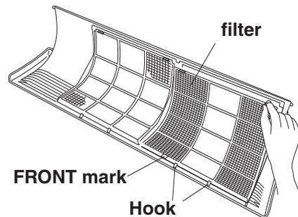
2. Allow the edge of the air intake grille to slide into the top of the indoor unit, and then insert it all the way inside.
