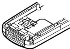
5. Hold the battery so that the metal contacts of the battery are facing down and the guides on the top of the battery slide into the battery slots ①, and then insert it ②.
