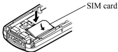
4. Slide the SIM lock lever to the right until the SIM is locked.
