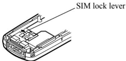
4. Remove the SIM card from the SIM holder.
