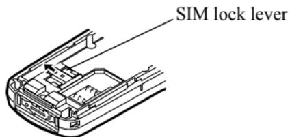
3. Position the SIM card with the gold contacts facing down, and slide the SIM into the SIM holder.
