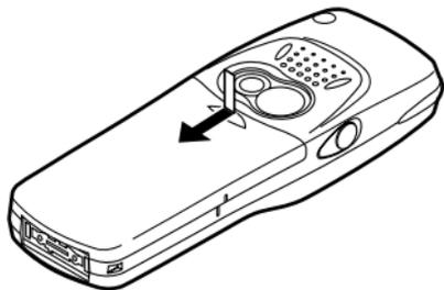
2. Pick up the battery using the protruding edge and remove the battery from the phone.
