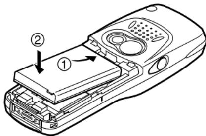
6. Replace the battery cover so that the marks are aligned and slide it as shown.
