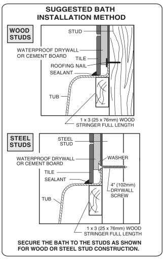
**C.)** Any finish material such as tile or wallboard must be self-supporting if it contacts the deck of the bath. Flooring will be butted against the bottom of the tub apron, also holding the tub in place.
