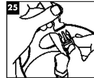
Clip tether from bottom of the Liberty power head around tank handle. Tighten securely making sure not to dislodge tank from cradle position.
