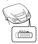
Slide HOLD in the direction of the arrow. When you press any button, "Hal d" appears in the display and you cannot operate the
