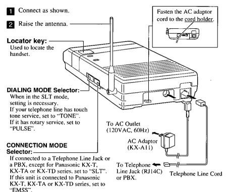
THE AC OUTLET POWER SOCKET SHOULD BE LOCATED NEAR THIS EQUIPMENT AND BE EASILY ACCESSIBLE.
