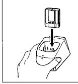
While holding the charging stand with one hand, push the battery in with the other hand until you hear a click.
