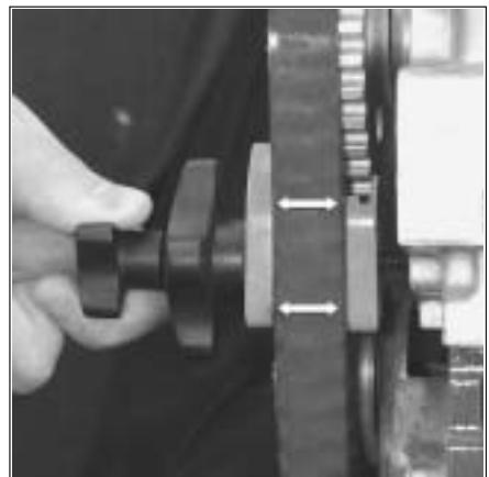
Clamp the Assembly onto the sprocket by screwing down the Large Locking Knob.
