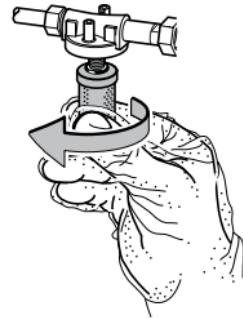
Wrap the used filter cartridge or the cleaning material in the safety glove to protect against odours and oil.
