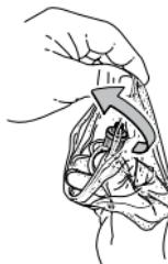
Hold new filter cartridge by the upper plastic part and **screw in by hand** (max. 1.5 Nm).
