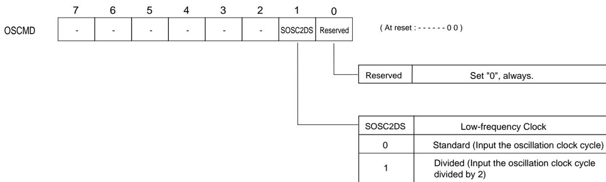
Figure 2-5-1 Oscillator Frequency Control Register (OSCMD : x'03F2D', R/W)
