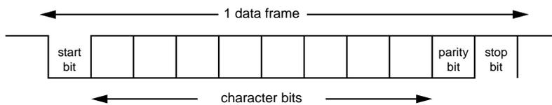
**Figure 11-3-15 UART Serial Interface Transmission / Reception Data Format**
