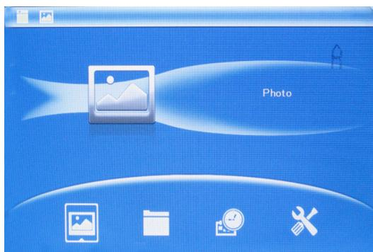
It supports SD/SDHC/MS/MMC and USB 2.0. After inserting a card or USB device, slideshow will play automatically, then press **EXIT** to access to Photo, File, Calendar and Setup interface. Press **▶||** to confirm.
