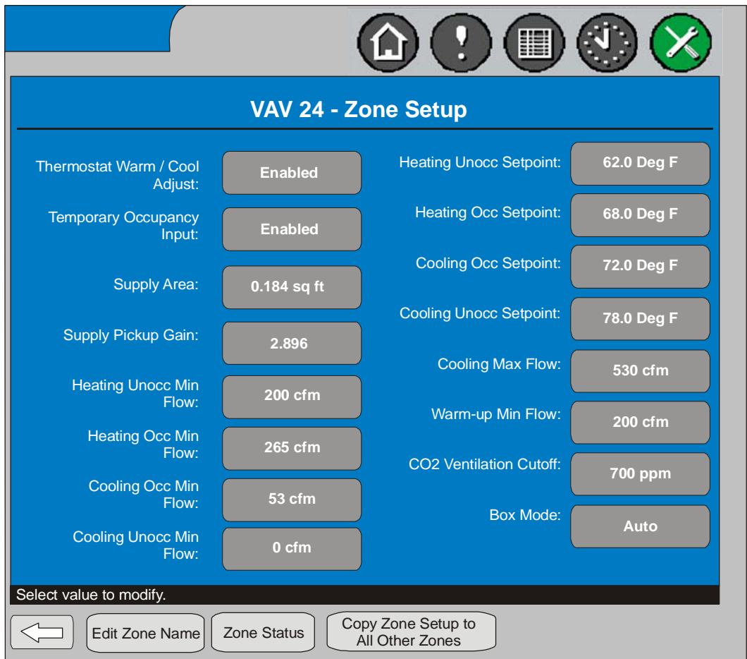
Figure 44: VAV RTU Zone Setup Screen
