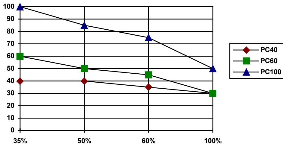
The graph shows the cutting current (in Amps.) on the Y axis and the percentage of working time calculated on a total time of 10 minutes on X axis.
