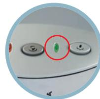
When the light switches on again, the machine is ready to begin dispensing steam.
