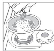
1. Remove the lower rack and unscrew the cap (anticlockwise).
