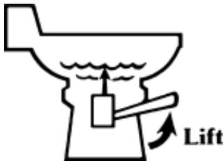
2. To flush toilet, press flush lever sharply down to the floor until contents clear bowl. A sharp popping noise is normal when the vacuum seal is broken and flushing action begins. Be sure to hold lever down for three seconds. If flush lever is accidentally released before waste clears bowl, do not attempt to flush toilet again until vacuum pump stops running. A small amount of water should remain in the bowl after flushing.
