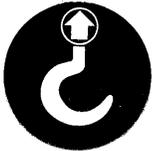
**Use approved safety straps or chains to lift the loader at the marked lifting points.**
