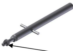
Unscrew and completely remove the standard threaded pin (2).
