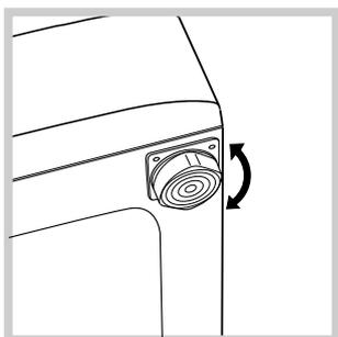
2. If the floor is not perfectly level, compensate for any unevenness by tightening or loosening the adjustable front feet (see figure); the angle of inclination, measured according to the worktop, must not exceed 2°.
