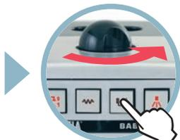
Turn the knob counter-clockwise and press the button.
