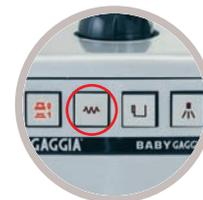
The machine is ready for use when the light goes off.
