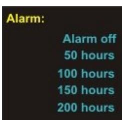
Setting the useful life of filters. This function enables to watch the life of the filters beginning at the moment of setting the value. This alarm is useful, for example, if there is a time limit for using a filter; e.g. for mercury filters it is only 50 hours.
