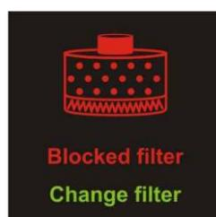
Alarm – alarm informing the user about unsatisfactory air-flow through the unit due to filter clogging. It is vital to leave the contaminated area and replace filters.
