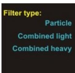
Filter type being used at present. **If the incorrect type of filter is set, the filter clogging control does not work correctly.**
