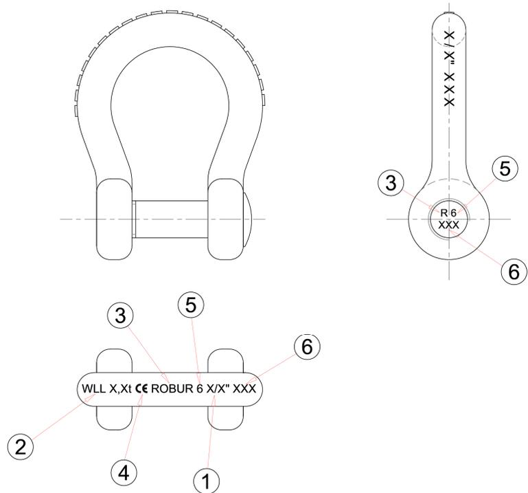
The position of the marking in the drawing is given purely as an indication. The various items may actually be found in different positions.
