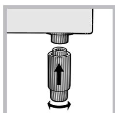
The legs\* fit into the slots on the underside of the base of the cooker.
