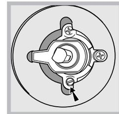
3. While the burner is alight, quickly change the position of the knob from minimum to maximum and vice versa several times, checking that the flame is not extinguished.
