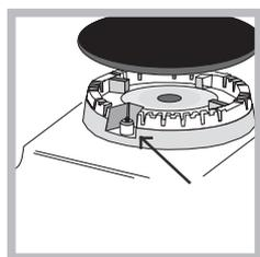
device\* (see figure), press the BURNER knob and turn it in an anticlockwise direction, towards the minimum flame setting, until the burner is lit. The burner may be extinguished when the knob is released. If this occurs, repeat the operation, holding
