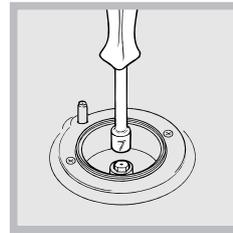
2. Unscrew the nozzles using a 7 mm socket spanner (*see figure*), and replace them with nozzles suited to the new type of gas (*see Burner and nozzle specifications table*).
