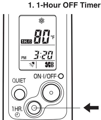
This function causes the unit to operate for one hour and then stop, regardless of whether the unit is on or off when this button is pressed. The **1HR.** indicator in the display indicates that this function is operating.
