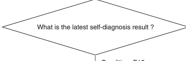
Condition: E01 → Defect in the inter-unit cable
