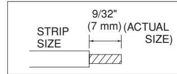
**Fig. 28****b) For Outdoor Unit****■ For solid core wiring (or F-cable)**
