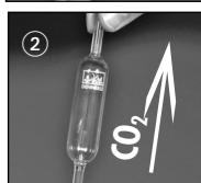
2. Connect check valve and bubble counter with a section of hose of around 5 cm in length. The outlet opening in the bubble counter must point in the direction of flow! ②
