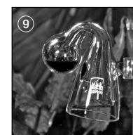
4. Carefully turn the test container around and use the suction clip to secure it in an upright position at a clearly visible point in the aquarium where a gentle flow of water prevails. ⑨
