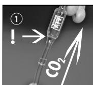
1. Connect CO<sub>2</sub> check valve to the supply hose of the CO<sub>2</sub> fertilizer system. The red tappet is ground on one side for sealing purposes. This point is indicated by a fine, white ring. This ring must always point towards the pressure reducer! ①
