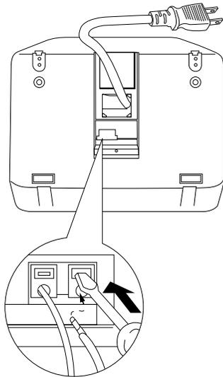
**2** Insert two wires for an external time signal while pushing the upper part of the terminal board with a screwdriver.
