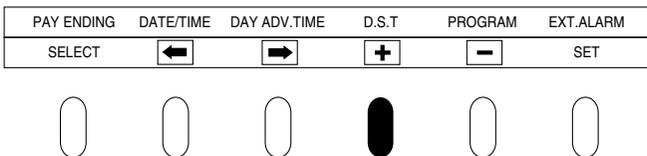
(2) Check the settings on the display and press **SET**. Now the setting is completed.
