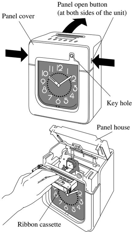
**1** Unlock the unit. While holding down the panel, open buttons at both sides of the unit, and lift the panel cover away from you.
