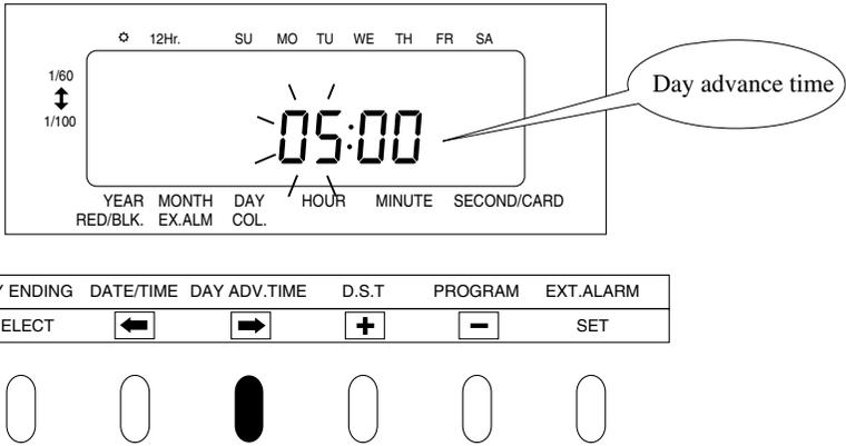
**2** Press **←** or **→** to cause digits to flash, and then press **+** or **-** to select the desired time.
