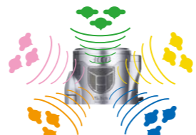
Five mics capture each of the sounds from the different sound source directions.
