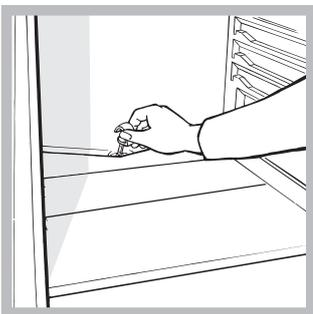
The refrigerator has an automatic defrosting function: water is ducted to the back of the appliance by a special discharge outlet (*see diagram*) where the heat produced by the compressor causes it to evaporate. It is necessary to clean the discharge hole regularly so that the water can flow out easily.
