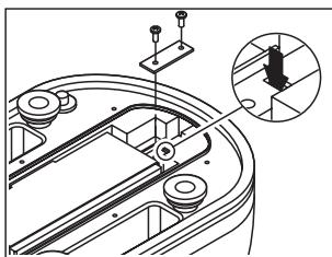
Use a small flat-tip screwdriver to short-circuit the two contacts in the rectangular opening (see arrow).
