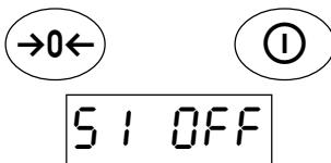
With the scale switched off, press the **→0←** key and hold it down. Switch on the scale with the **1** key.
