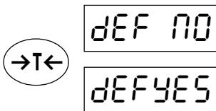
The factory settings can only be restored in **service mode** in the menu block "DEF" ("Default"). If you want to restore the factory settings, select "DEF YES" and confirm with the ① key. Then press the →0← key and confirm the "SAVE" prompt with the ① key. **Note: When the factory settings are restored, all individual settings are lost!**
