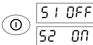
Press the ① key to confirm the setting in the current menu block and then select the next menu block.
