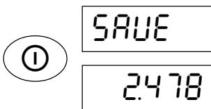
If you want to save the settings, press the ① key. When the save has been done, the scale automatically returns to weighing mode.
