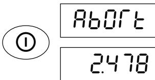
If you do not want to save your changes, press the →T← key. The display shows "Abort". Press the ① key and the scale returns to weighing mode without the changed settings being saved.
