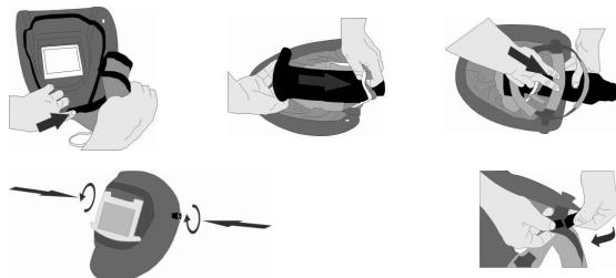
**For hygiene reasons, discard the old face seal immediately after replacement so that it cannot be reused. The face seal must not be washed! Washing causes loss of the protective impregnation securing incombustibility!!!**
