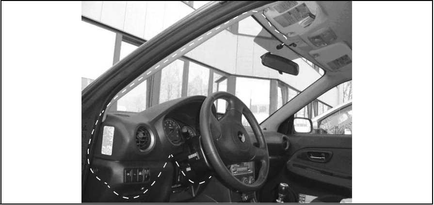
Illust. 4: Route sensor connecting wire.
