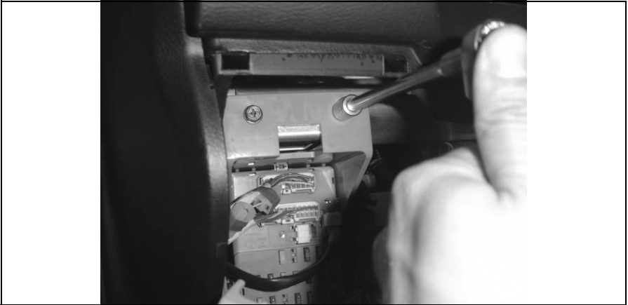
Illust. 5: Fix relay holder with screws
