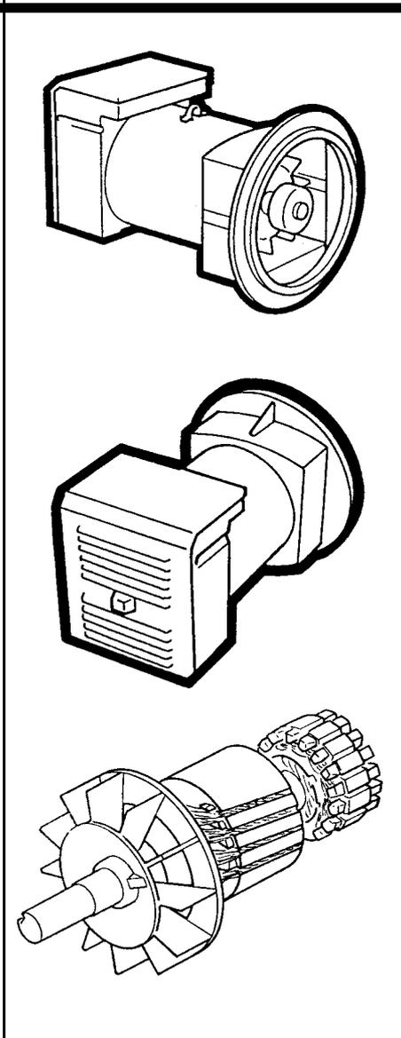
ECO3-N 2 and 4 pole alternators are brushless, self regulating and incorporate a rotating inductor with damper cage (2 pole generators) and a fixed stator with skewed slots. The stator windings have a shortened pitch to reduce the harmonic content of the output waveform.
