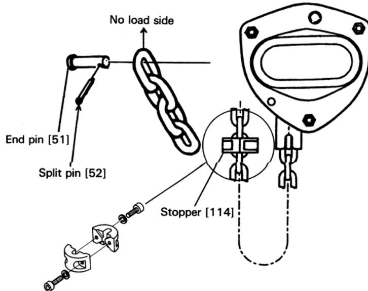
**Figure 6-8 10 Ton & Above Anchorage Assembly**
