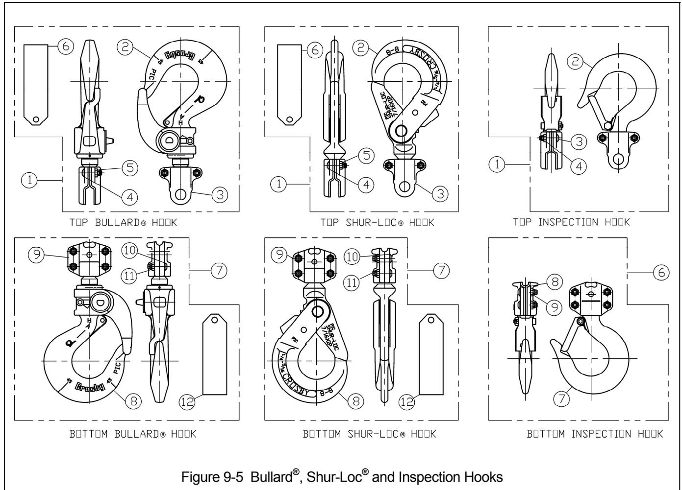
Figure 9-5 Bullard®, Shur-Loc® and Inspection Hooks
