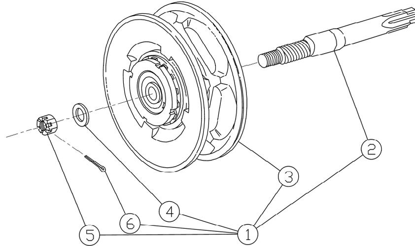
Figure 9-4 Slip Clutch
