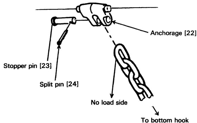
Figure 6-7 8 Ton & Below Anchorage Assembly
