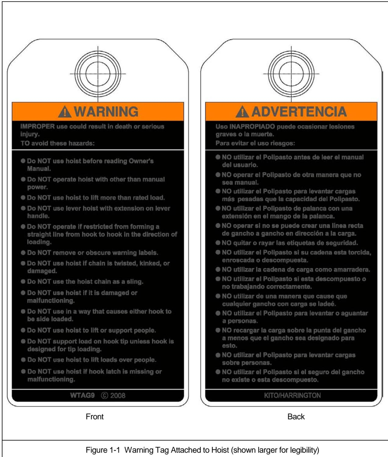
Figure 1-1 Warning Tag Attached to Hoist (shown larger for legibility)
