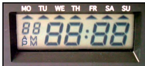
Figure 6-4. LCD Test Display.
