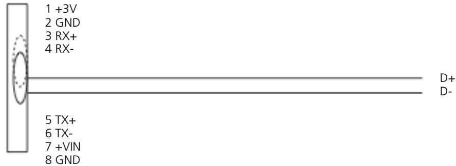
Figure 3-3. RS-485 wiring diagram for LES1102A.
