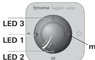
If the unit is switched on using this pushbutton, the system is automatically reset to the factory settings (COOL, FAN HIGH, TEMP. 21 °C).
