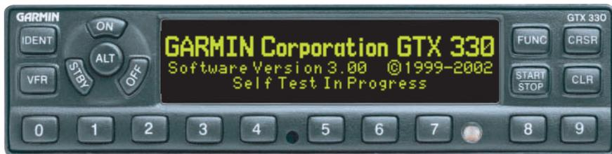
The GTX 330 transponder is powered on by pressing the **STBY**, **ALT** or **ON** keys, or by a remote avionics master switch (if applicable). After power on, a start-up page is displayed while the unit performs a self test. (See your Garmin dealer for software upgrades.)
