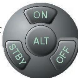
Any time the function **ON** or **ALT** is selected the transponder becomes an active part of the Air Traffic Control Radar Beacon System (ATCRBS). The transponder also responds to interrogations from TCAS equipped aircraft.
