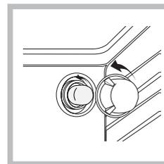
2. Unscrew the light bulb and replace it with a similar one: voltage 230 V, wattage 25 W, cap E 14.
