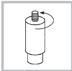
If it is necessary to level the appliance, screw the adjustable feet into the places provided on each corner of the base of the cooker (*see figure*).
