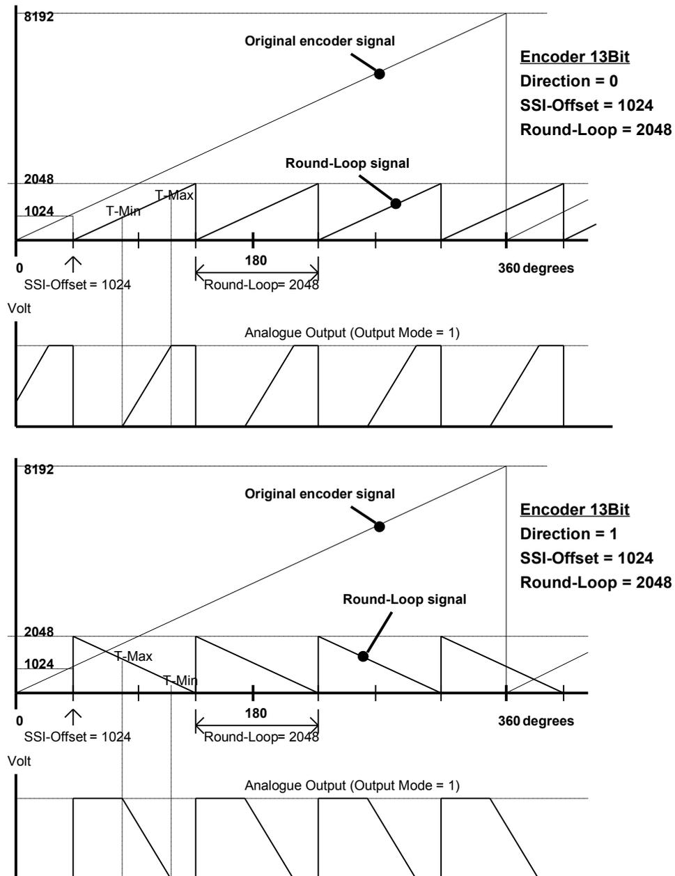
The ROUND LOOP function is also suitable for suppression of the encoder overflow, when the mechanical zero position of your encoder is found between your **Teach Minimum** and **Teach Maximum** values and you do not like to change the mechanical configuration. As shown in the subsequent Figure, you
