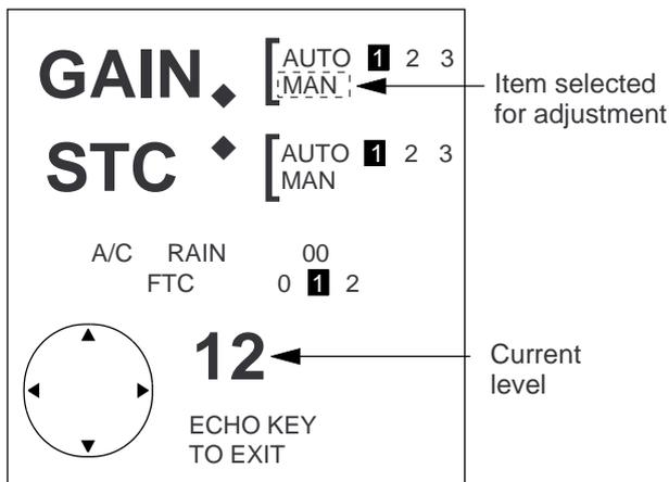
Figure 2-4 Display for adjustment of GAIN, STC, A/C RAIN and FTC
