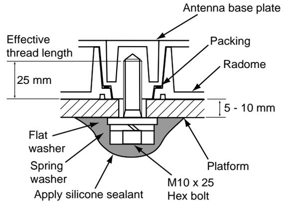
Figure 5-5 How to fasten the radome base to the mounting platform
