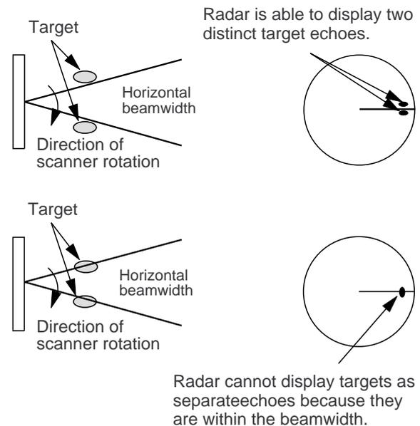
Figure 3-3 Bearing resolution
