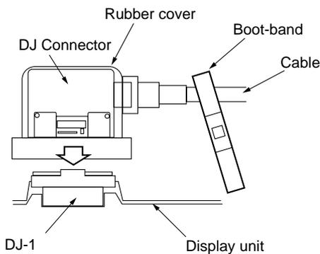
2. Cover the connector with the rubber cover. The projection on the connector base is inserted into the groove on the rubber cover.
