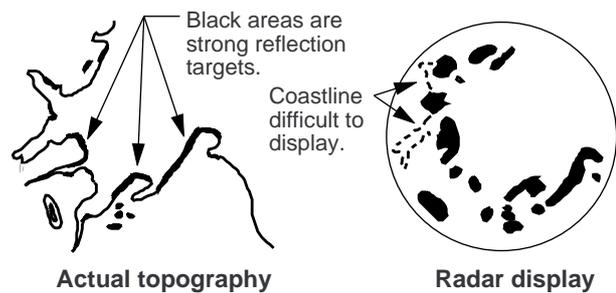
Figure 3-8 Nautical chart and associated radar picture
