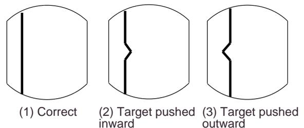
*Figure 5-19 Examples of improper and correct sweep timings*
