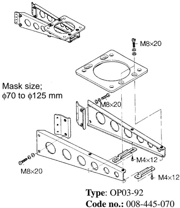
Figure 5-3 Assembling the sailboat mast mounting bracket (option)
