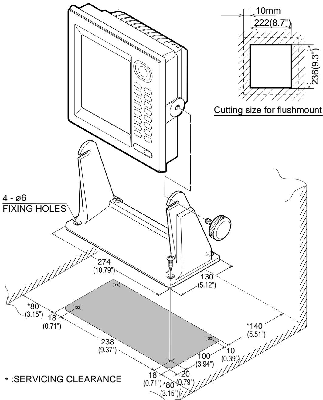
Figure 5-11 How to mount the display unit
