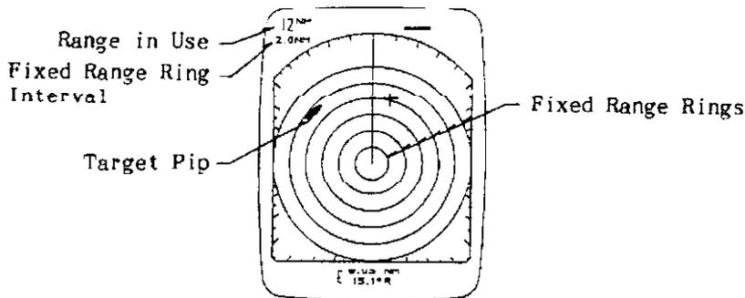
Fig.26 Range Measurement with the Fixed Range Rings
