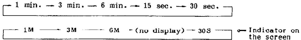
Press the PLOT touchpad again after 10 seconds passed, and the plot function is canceled and the normal radar picture is restored.
