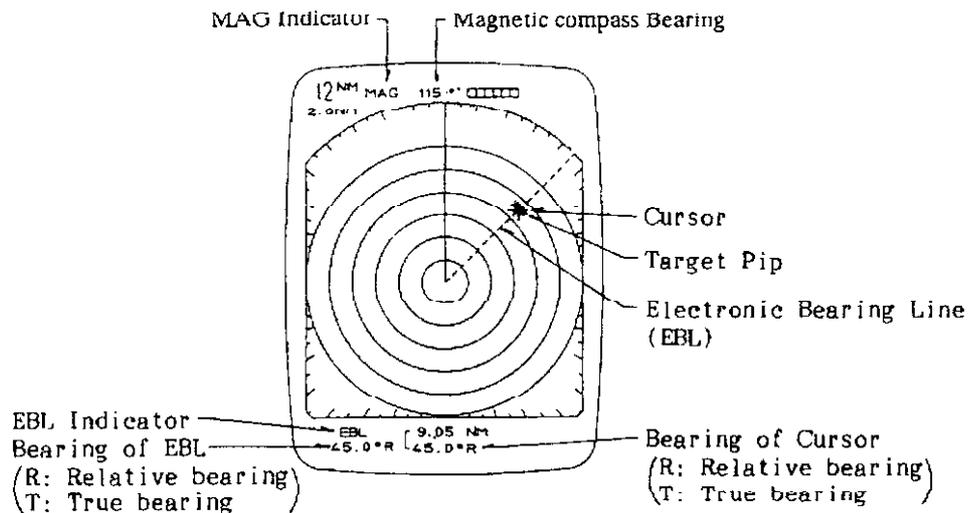
Fig.28 Bearing Measurement with the "+" Cursor and the EBL
