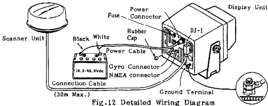
Fig.12 Detailed Wiring Diagram
