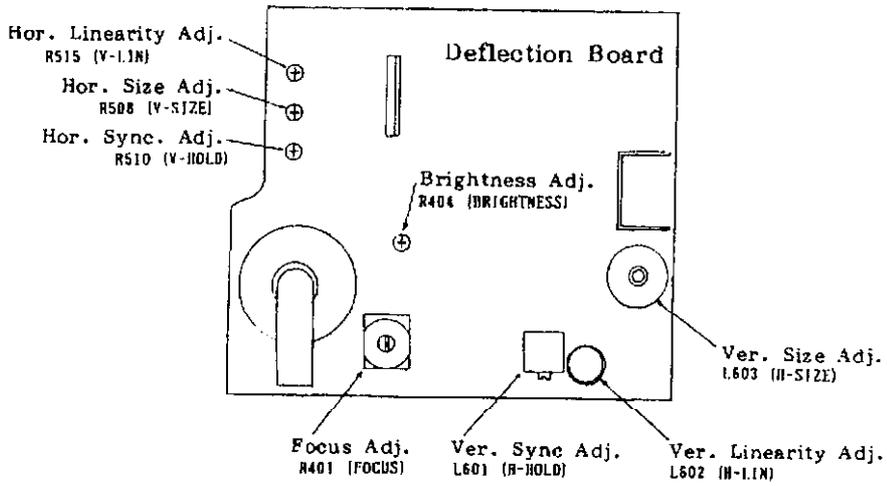
Note: Since the CRT is turned 90°, the indications "V" and "H" correspond to "horizontal" and "vertical", respectively.
