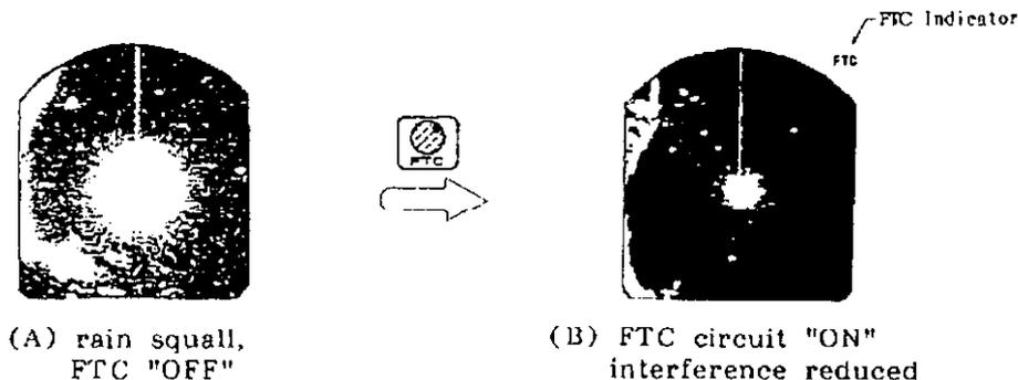
Fig.29 Precipitation Interference
