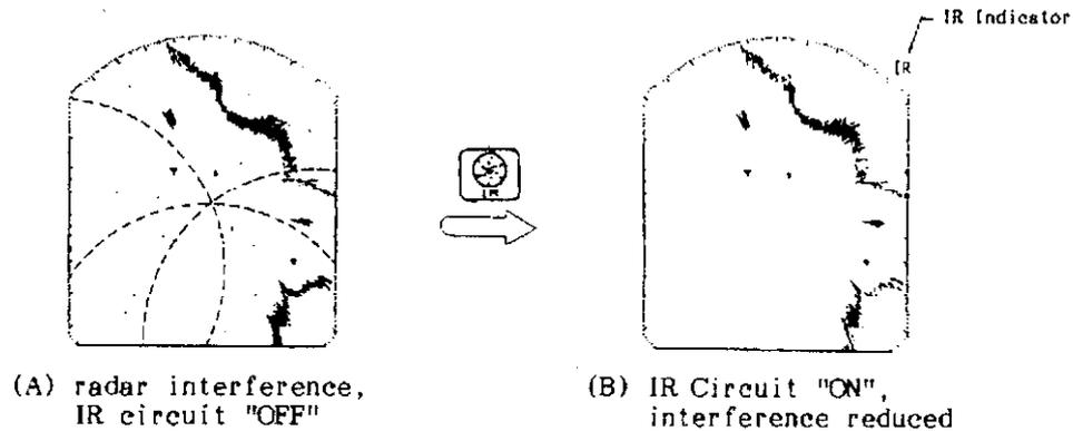
Fig.30 Radar Interference
