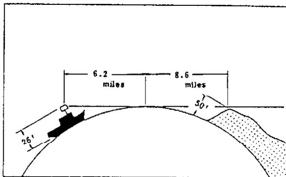
Fig.38 Radar Horizon
