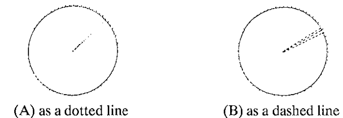
Fig.3-14 Ramark Signal Appearance
