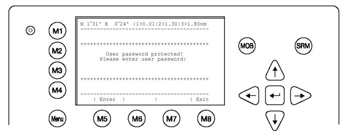
Scroll to the Voyage Setting Fields with up and down arrows and input your vessel data. Select a default Cargo Type, Draught, POB (Persons on board), Destination, ETA and Navigation Status Setting using the [Left] & [Right] arrow keys.
