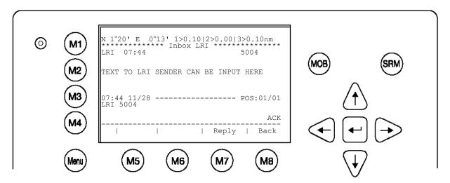
An LRI has arrived; the NAUTICAST Settings are configured to **Manual Mode**: The LRI therefore needs to be manually handled (accepted or rejected)
