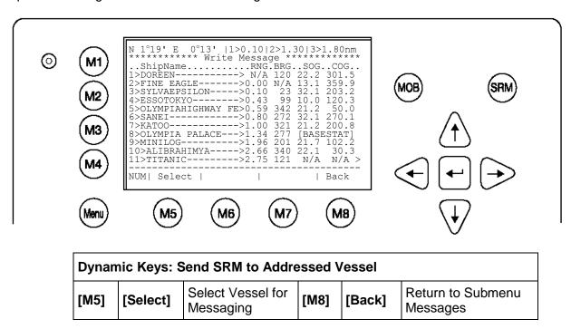
**NOTE**: The SRM message transmission is automatically repeated every 180 seconds until the [Stop] button has been pressed.
