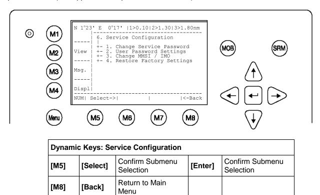
After entering the Default Service Password in the password query, the Service Configuration Menu may be accessed. In this menu it is possible to configure both the Service Password and the User Password Settings, as well as input the MMSI/IMO Numbers and reset them to Factory Settings.
