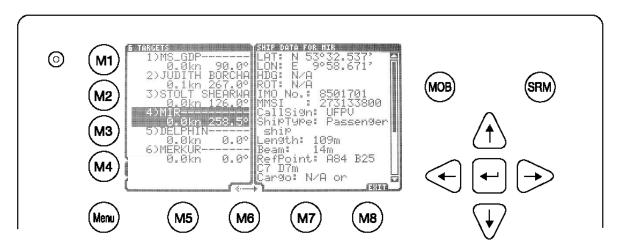
Pressing [Up] or [Down] scrolls the ship detail list by line, [Left] or [Right] by page. [M8] returns to the minimized view.
