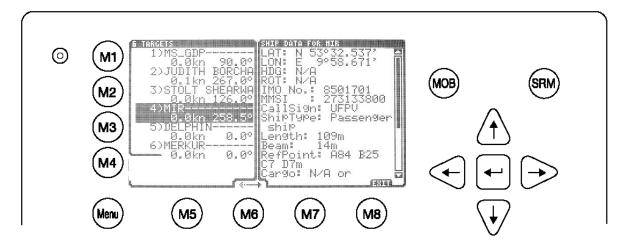
Pressing [Up] or [Down] scrolls the ship detail list by line, [Left] or [Right] by page. [M8] returns to the minimized view.
