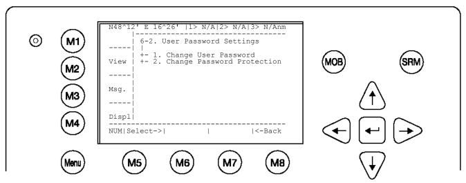
Enter the new Password. A minimum of 6, a maximum of 8 characters are allowed. Should the new password include numbers, use the shift key to generate them.
