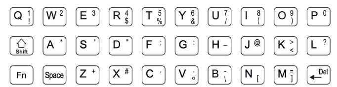
Tip: The NAUTICAST automatically changes the keys "Q" through to "P" to numerical input when the current application requires numbers, rather than letters to be input. This feature is enabled when [NUM] appears on the bottom left hand side of the screen.
