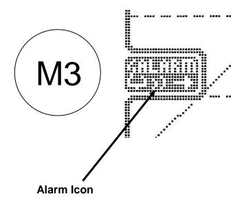
Pressing the [M3] button shows the details of the selected alert.
