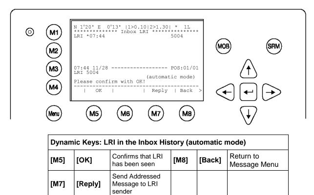
Upon activation of the [OK] button, the user confirms that he has been notified of a current Transponder system interrogation. This information is useful, as it prevents unknown interrogation from taking place when the transponder is set in automatic mode.
