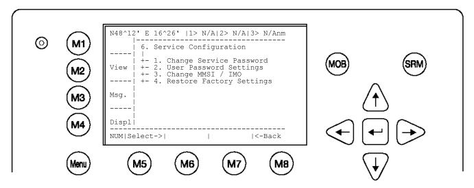
Select Submenu 1 "Change User Password" with cursor button [Up] & [Down] by pressing Number 1 on the keyboard.
