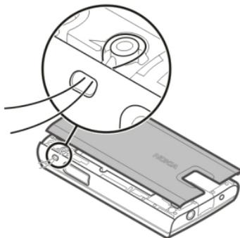
Thread a strap as shown in the picture and tighten it.
