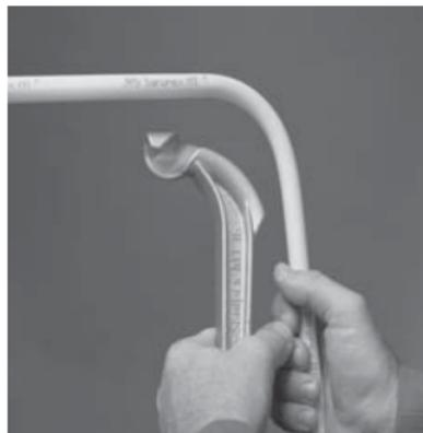
Remove the completed pipe bend from the manual bending template.
