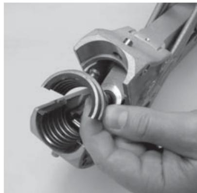
By pressing the upper or lower release pin, the respective clamping jaws (2) are released. Remove the clamping jaws via guidance and insert the desired clamping jaws until the snap.
