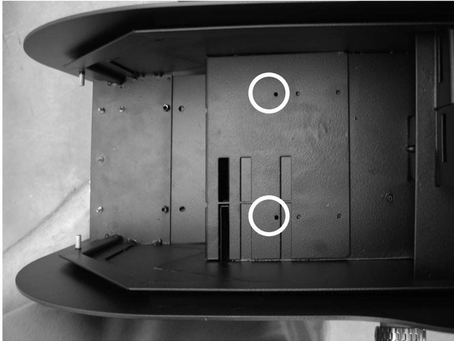
If an NV8/NV10 banknote validator is installed, make sure that the partition is positioned in the most retracted position possible and that it is fixed using the holes indicated in the figure.
