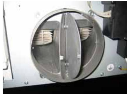
In filtering application that the stop valve doesn't permit the entrance of wind and exhausted air.
