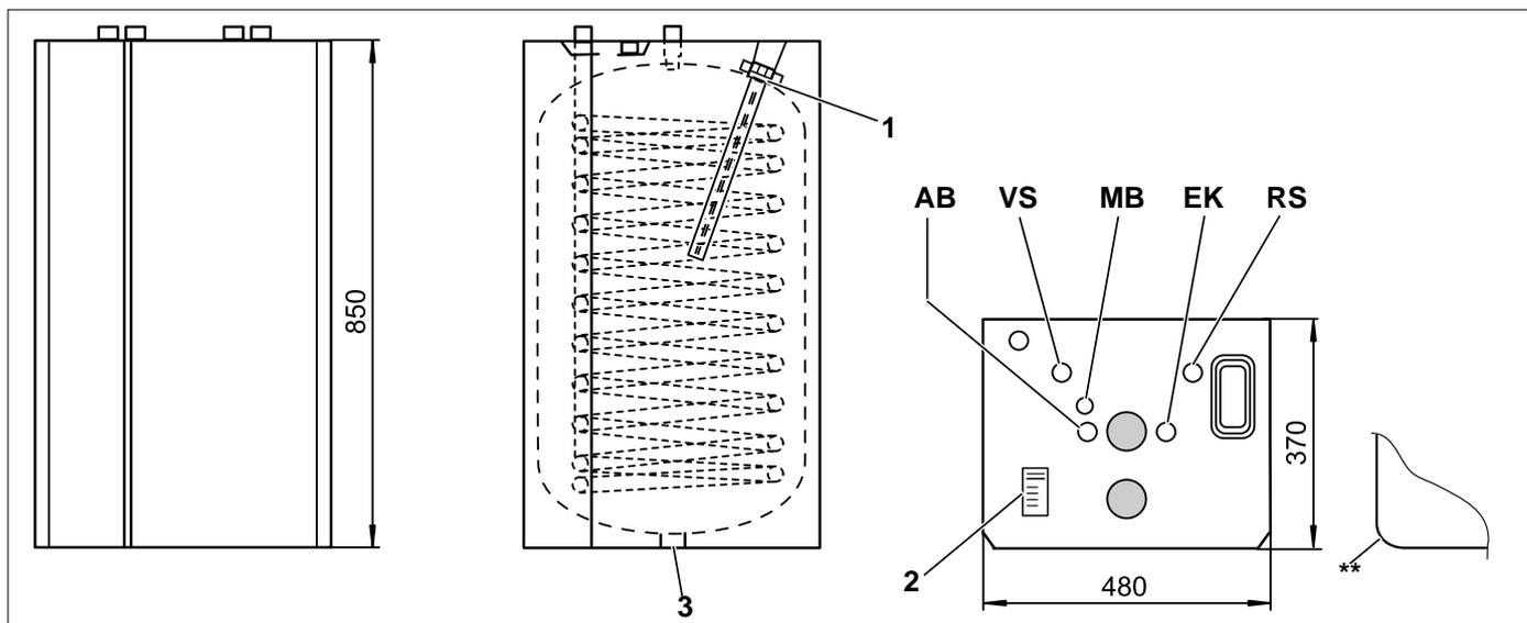
Fig. 1 Dimensioni Logalux HT 70 W/H 70 W
