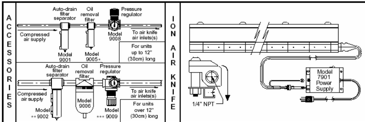
\* Use Model 9006 Oil Removal Filter for Ion Air Knives longer than 6" (15cm)
