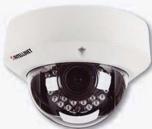
**IDC-757IR Pro-Level Indoor/Outdoor Night Vision Megapixel Network Dome Camera. 720p HD, WDR, Day/Night, IP66, H.264, MPEG4, M-JPEG, 3GPP, PoE, MicroSD/SDHC.**
