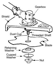
NOTE: Make sure all parts are in place as illustrated, and the blade is sandwiched between the dust cup and the retaining washer. There should be no space between the blade and the dust cup or the retaining washer.
